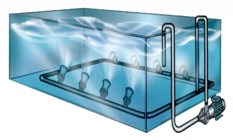
Innovative AIR-LESS® eductor agitation for a safer working environment. Undoubtedly the most cost effective alternative to traditional air agitation.
